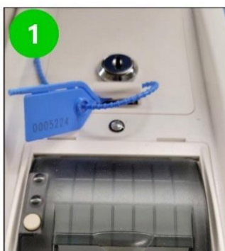
Seal numbers from blue security seals installed on both vDrive compartments after removal of the vDrives.
