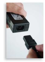
Plug the power brick into the back of the Verity Scan (flat part up). ▼
