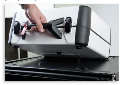
Reach inside the ballot box and push the latch away from you to lock the lid and the Verity Scan in place.
