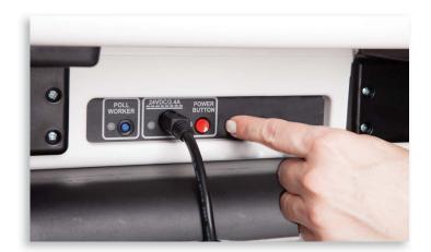
During the power on process, the Verity Scan will print the Power-On Self Test report on its built-in thermal printer. This report will indicate any hardware or connection issues; if any issues are noted, check connections and restart the device using the red power button.
