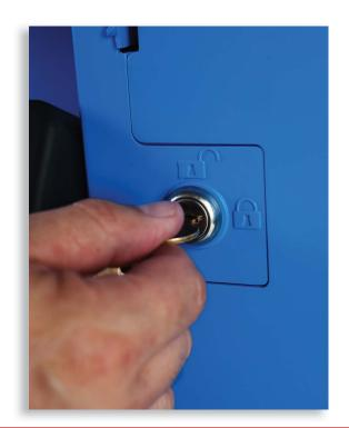
! IMPORTANT: Verity Scan will not function unless the lock is engaged.
