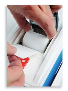
Close the printer cover. The paper must extend out from underneath the front edge of the cover. The white button can be used to advance the paper.
