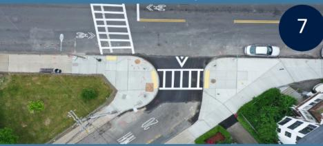
Curb or sidewalk extended into the street, either at an intersection or mid-block, narrows the street width, reduces pedestrian crossing distance, improves visibility of pedestrians, and reduces right-turning vehicle speeds.
