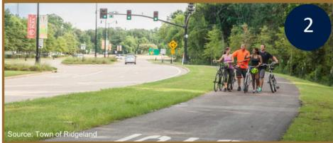
This facility is shared between people biking and walking. A shared use path (SUP) or trail provides the highest level of separation and the lowest level of traffic stress for cyclists.
