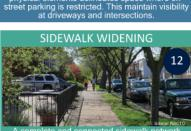
A complete and connected sidewalk network increases pedestrian access and safety. Along an urban corridor, the sidewalk clear width should be at least 6-ft wide, or ideally wider.
