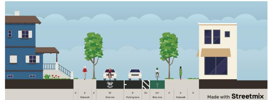
*Contra-Flow Bike-Lane with On-Road Shared Lane Marking and Sidewalk, Cross-Section. (Image credit: Streetmix.net, TPD) See also – Segment D, Cross Sections #2 & #3, earlier in this chapter.*
