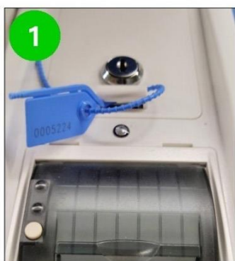
Blue Security Seals from both vDrive Compartments. DO NOT REMOVE UNTIL POLLS CLOSE
