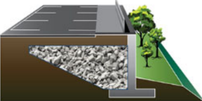
Retaining Walls & Bridge Abutments
