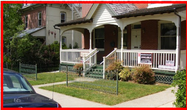
Bad example of front facade with inappropriate location, scale, and materials of signs and fencing to the historic setting
