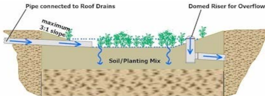
Figure B-5: Typical Rain Garden/Bioretention Area
