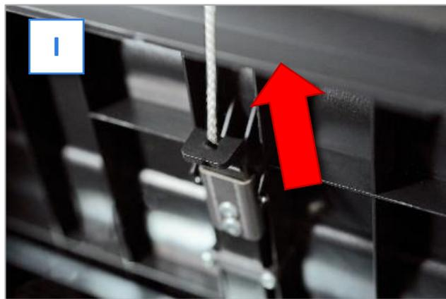
8. Lift the lid while gently pulling upward and outward, ensuring that the double hinge is fully extended. Lay the lid across the top of ballot box and press it down. Do **NOT** force it. Instead drop the lid back down to release the double hinge and try again [J, K, L] ▼
