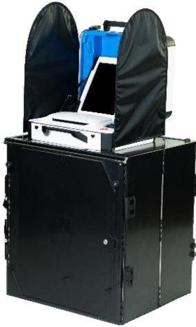
The scanner is a polling place-based digital scanner for scanning and casting paper ballots.
